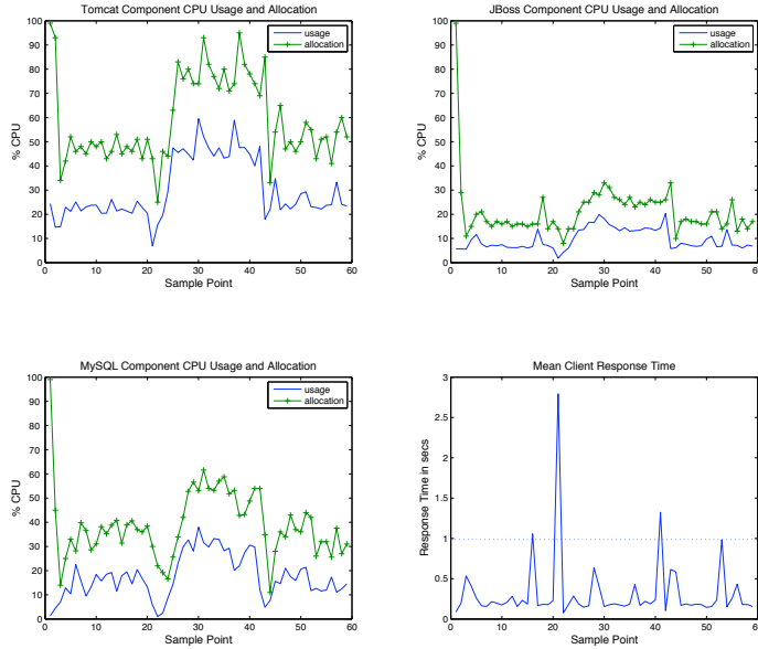
Fig. 4. MIMO Controller CPU allocation and measured mRT.
